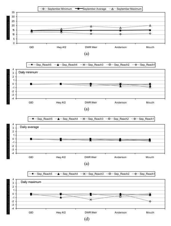
**Figure 5-41** Shadinge Study results for September. Deviations from (a) September base-case condition in (b) daily minima, (c) daily average, and (d) daily maxima of simulated water temperature at GID, Hwy 12, DWR Weir, Anderson Grade Road, and the mouth of the Shasta River.
