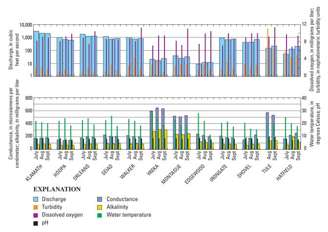
**Figure 9.** Monthly water-quality sampling data for July, August, and September 2002 for six sites on the Klamath River, one site on the Trinity River, three sites on the Shasta River, and two sites on the Lost River in the Lower Klamath River Basin, Califonia. *A.* Instantaneous discharge, dissolved oxygen (DO), and turbidity, and *B.* Specific conductance, alkalinity, water temperature, and pH.
