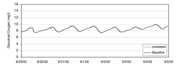
Figure 50. Dissolved oxygen at Mouth, PFAC = 1.25: 8/29/02 to 9/5/02
