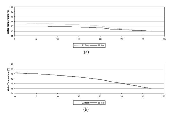
Figure 4-8 Longitudinal profile of average daily temperature for August 28, 2001 meteorological conditions for 50 cfs test case with varying tree height, (a) tr=50% (b) tr=85%
