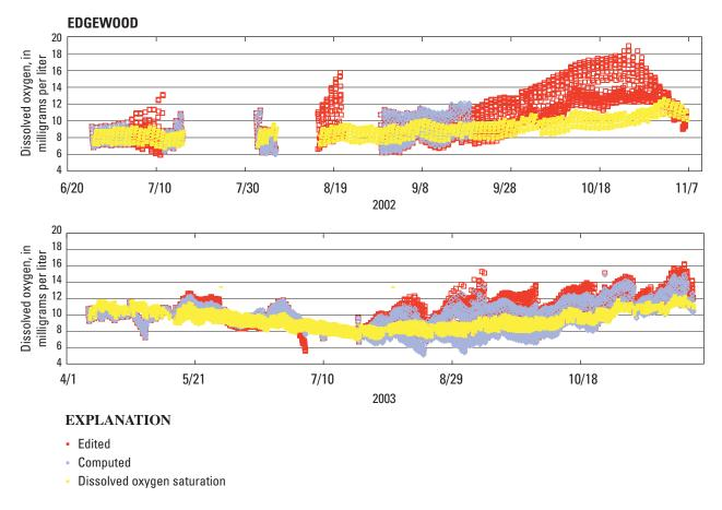
**Figure A2-1.** Measured continuous data of dissolved oxygen with initial edited record, computed record, and saturated values for 2002 and 2003 for USGS sites on the Shasta River, (*A*) EDGEW00D, (*B*) MONTAGUE, (*C*) HWY3, and (*D*) YREKA.
