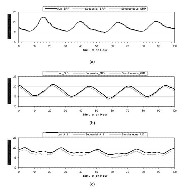
Figure 5-30 Time series from day 1 through 4 of the baseline, sequential, and simultaneous pulse flows for (a) SRP, (b) GID, (c) A12, (d) DWR, (e) AND, and (e) MOU locations. Continued on next page.
