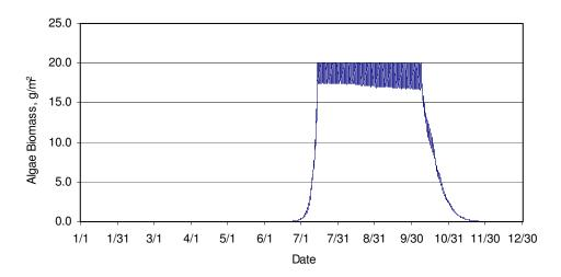
Figure 48. Algal biomass with global shade factor equal to 0.9
