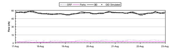
Figure 5-1 Measured vs. simulated flow for GID, Aug 17-Aug 23, 2001
