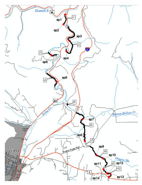
Figure 1a. Shasta River survey reaches and sample points – mouth to Highway 3.
