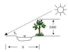
Figure 2-2 Diagram depicting the variables for calculating X, the length of the shadow parallel to the azimuth of the sun
