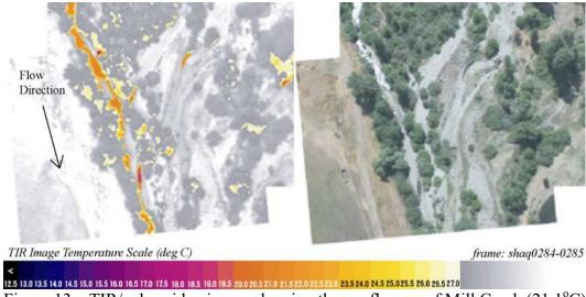
Figure 13 – TIR/color video image showing the confluence of Mill Creek (21.1°C) and the dry channel of Shackelford Creek at river mile 2.8. Small cool water seeps are visible in the TIR images suggesting at least some level of sub-surface exchange in the channel.
