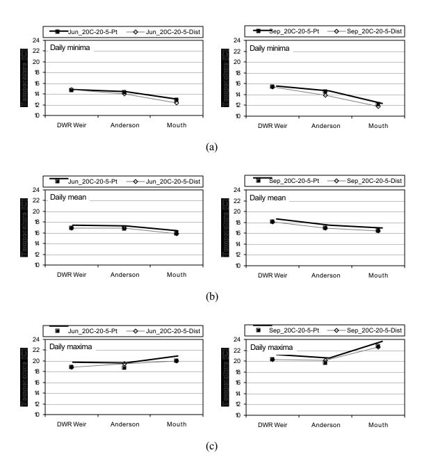
**Figure 5-35 Tailwater Return Study 20°C-20-5 results for June and September.** Upstream boundary condition of 20°C and 20 cfs at SRP, tailwater return flow of 5 cfs. Simulated (a) daily minimum, (b) daily average, and (c) daily maximum water temperature at DWR Weir, Anderson Grade Road, and the mouth of the Shasta River comparing point and distributed discharge of tailwater. Simulations designated by "month\_upstream water temperature-upstream inflow-tailwater flow" (e.g. Sep\_20C-20-5).
