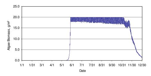
Figure 43. Algal biomass with maximum algal growth rate equal to 1.3 1/day
