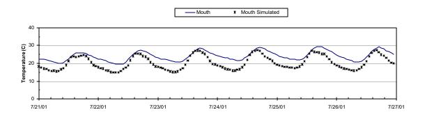
Figure 5-22 Measured vs. simulated temperature for Mouth, July 21-27, 2001
