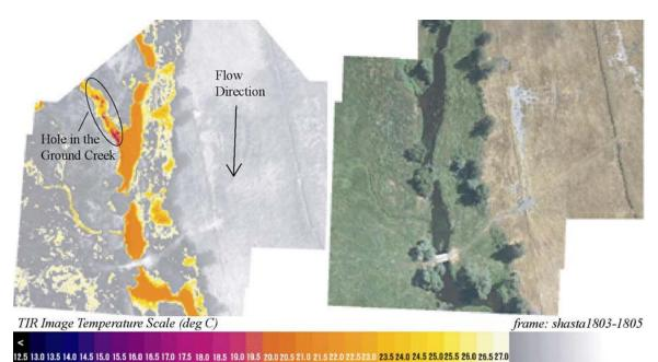
TIR/color video image pair showing the confluence of Hole in the Ground Creek  $(17.3^{\circ}C)$  to the right bank of the Shasta River  $(21.6^{\circ}C)$  at river mile 34.7.
