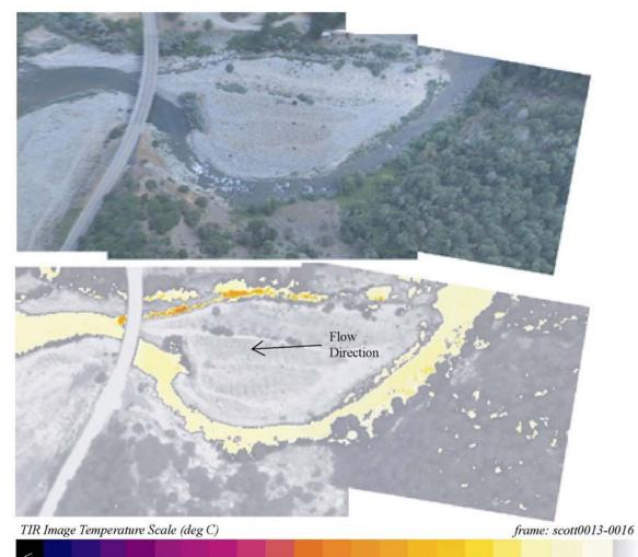
**17.0 17.5 18.0 18.5 19.0 19.5 20.0 20.5 21.0 21.5 22.0 22.5 23.0 23.5 24.0 24.5 25.0 25.5 26.0 26.5 27.0** TIR/color video image pair showing a spring  $(22.1^{\circ}C)$  in the side channel on the right bank of the Scott River  $(25.9^{\circ}C)$  at river mile 0.2.
