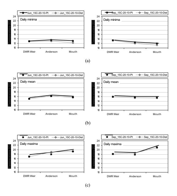
**Figure 5-32 Tailwater Return Study 15°C-20-10 results for June and September.** Upstream boundary condition of 15°C and 20 cfs at SRP, tailwater return flow of 10 cfs. Simulated (a) daily minimum, (b) daily average, and (c) daily maximum water temperature at DWR Weir, Anderson Grade Road, and the mouth of the Shasta River comparing point and distributed discharge of tailwater. Simulations designated by "month\_upstream water temperature-upstream inflow-tailwater flow" (e.g. Sep\_15C-20-10).
