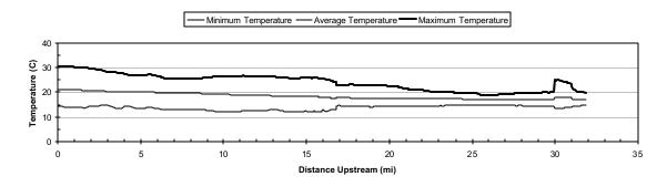
Figure 5-45 Simulated average, minimum, and maximum temperature: full riparian vegetation restoration between RM 34 and RM 17, with existing conditions from RM 17 to RM 0
