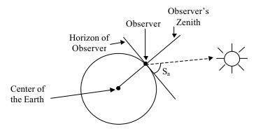
Figure 2-1 Diagram of the solar altitude
