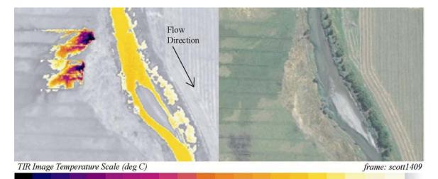
**17.0 17.5 18.0 18.5 19.0 19.5 20.0 20.5 21.0 21.5 22.0 22.5 23.0 23.5 24.0 24.5 25.0 25.5 26.0 26.5 27.0** TIR/color video image pair showing a thermal signature in a field near right bank of the Scott River (24.5 °C) at river mile 36.5. This thermal signature is presumed due to transpiring vegetation from irrigation or recent rain.
