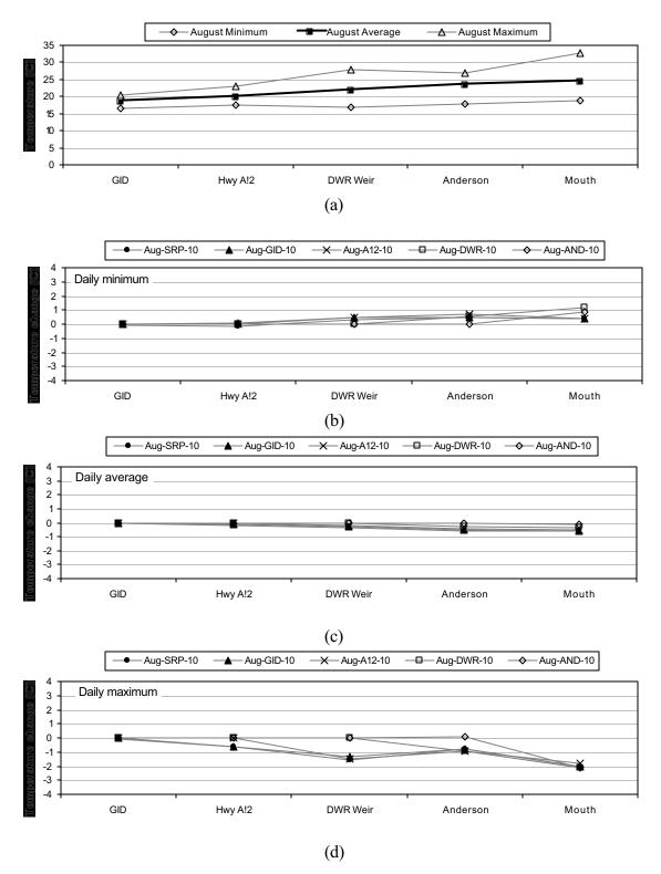
**Figure 5-25** Flow Regime Study results for 10 cfs inflows in August. Deviations from (a) August basecase condition in (b) daily minima, (c) daily average, and (d) daily maxima of simulated water temperature at GID, Hwy 12, DWR Weir, Anderson Grade Road, and the mouth of the Shasta River.
