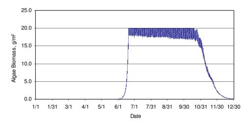
Figure 42. Algal biomass with maximum algal growth rate equal to 1.1 1/day
