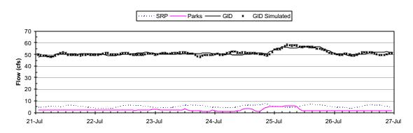
Figure 5-6 Measured vs. simulated flow for GID, July 21-July 27, 2001
