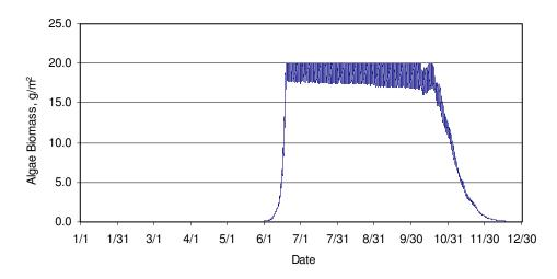
Figure 47. Algal biomass with global shade factor equal to 0.7
