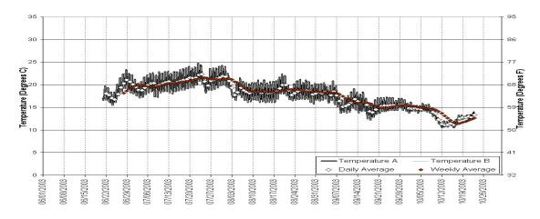
Figure 46. Continuous Temperature Data - Shasta River @ County Road A-12 - Collected by NCRWQCB: 06/01/03 - 10/31/03. (For quality control purposes, two optic StowAway sensors ( A and B ) were deployed at this site).
