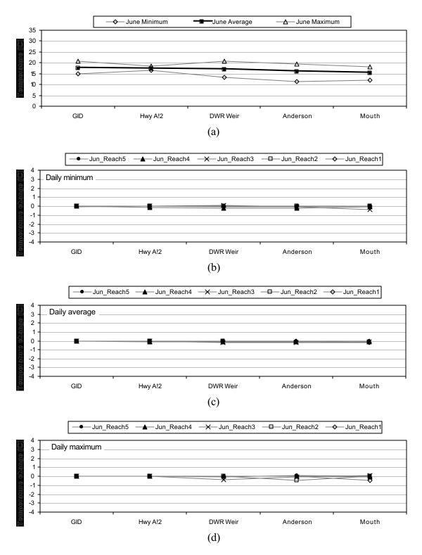
**Figure 5-39 Shadinge Study results for June.** Deviations from (a) June base-case condition in (b) daily minima, (c) daily average, and (d) daily maxima of simulated water temperature at GID, Hwy 12, DWR Weir, Anderson Grade Road, and the mouth of the Shasta River.
