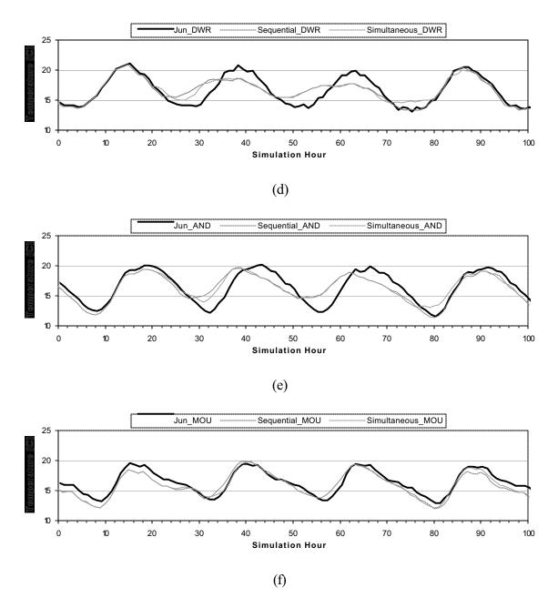
Figure 5-30, continued. Time series from day 1 through 4 of the baseline, sequential, and simultaneous pulse flows for (a) SRP, (b) GID, (c) A12, (d) DWR, (e) AND, and (e) MOU locations.
