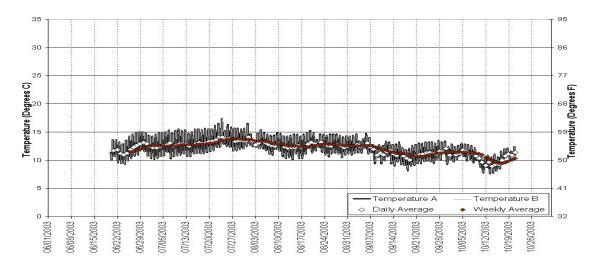
Figure 53. Continuous Temperature Data – Boles Creek - Collected by NCRWQCB: 06/01/03 - 10/31/03. (For quality control purposes, two optic StowAway sensors ( A and B ) were deployed at this site).
