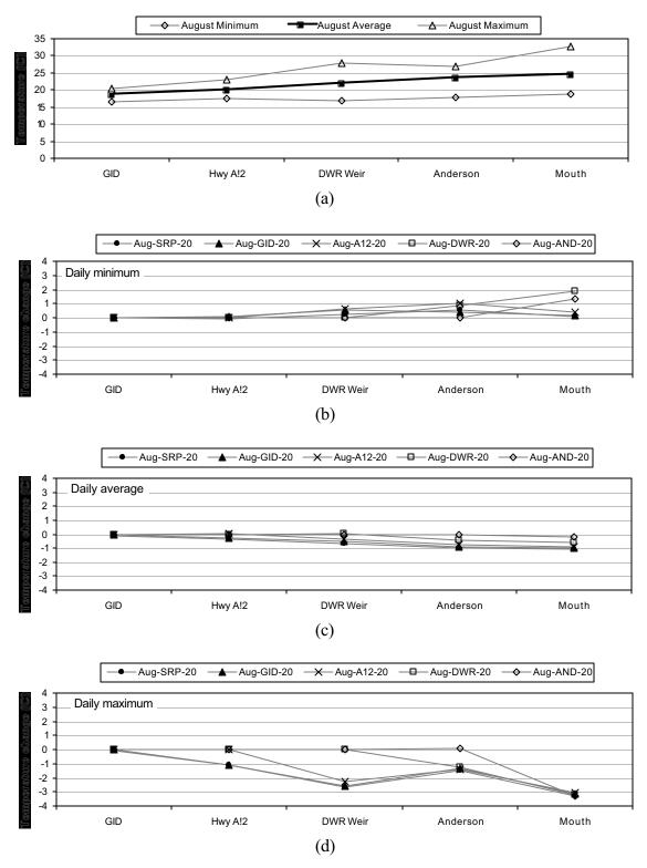
**Figure 5-26 Flow Regime Study results for 20 cfs inflows in August.** Deviations from (a) August basecase condition in (b) daily minima, (c) daily average, and (d) daily maxima of simulated water temperature at GID, Hwy 12, DWR Weir, Anderson Grade Road, and the mouth of the Shasta River.
