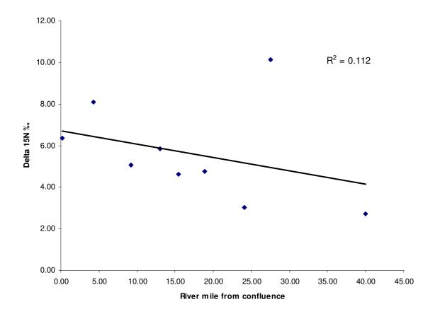
Figure 5. Suspended organic material stable nitrogen isotope values plotted against river mile for the Shasta River. River mile 0 is the confluence with the Klamath River. The single outlier point at river mile 27.49 is omitted from the plot.
