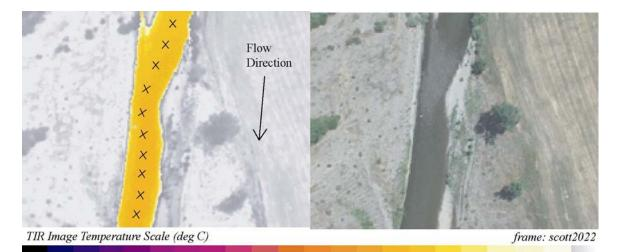
**17.0 17.5 18.0 18.5 19.0 19.5 20.0 20.5 21.0 21.5 22.0 22.5 23.0 23.5 24.0 24.5 25.0 25.5 26.0 26.5 27.0** Figure 1 – TIR/color video image pair showing how temperatures are sampled from the TIR images. The black X's on the TIR image show typical sampling locations near the center of the stream channel. The recorded temperature for this image is the median of the sample points.
