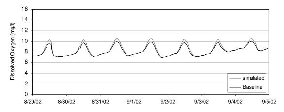
Figure 49. Dissolved oxygen at Anderson Rd, PFAC = 1.25: 8/29/02 to 9/5/02
