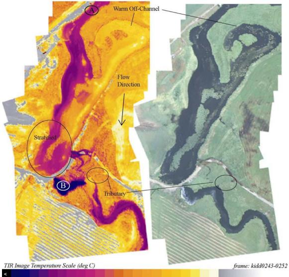
23.0 23.5 24.0 24.5 25.0 25.5 26.0 26.5 27.0 27.5 28.0 28.5 29.0 29.5 30.0 30.5 31.0 31.5 32.0 32.5 33.0 33.5 34.0 TIR/color video image pair showing a stratified stretch of Big Slough with an unnamed warm tributary  $(32.0^{\circ}C)$  on the left bank, in the bottom half of the image. The temperature at point A is 25.4°C while the temperature directly downstream of the bridge (B) is 23.9°C (river mile 6.0).
