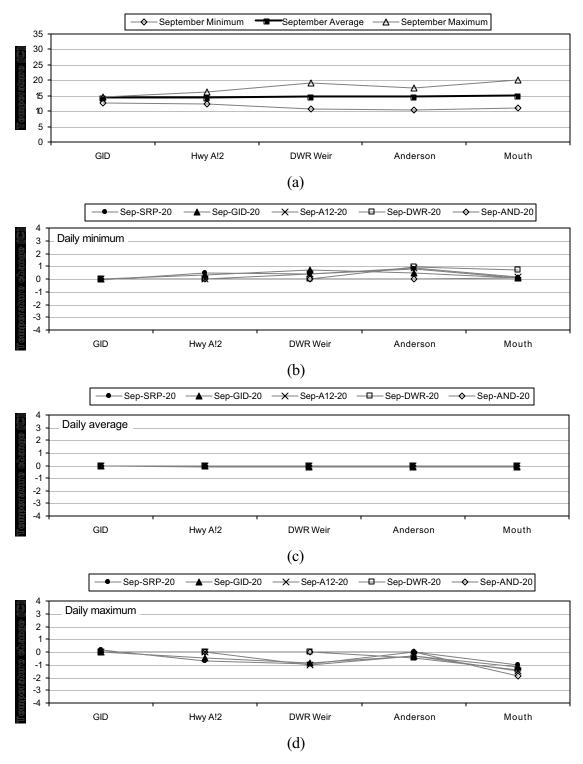
**Figure 5-28 Flow Regime Study results for 20 cfs inflows in September.** Deviations from (a) September base-case condition in (b) daily minima, (c) daily average, and (d) daily maxima of simulated water temperature at GID, Hwy 12, DWR Weir, Anderson Grade Road, and the mouth of the Shasta River.
