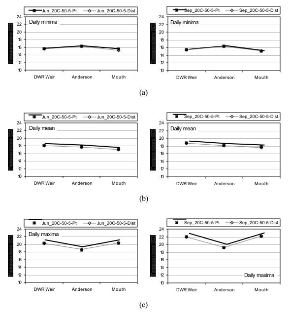
**Figure 5-37 Tailwater Return Study 20°C-50-5 results for June and September.** Upstream boundary condition of 20°C and 50 cfs at SRP, tailwater return flow of 5 cfs. Simulated (a) daily minimum, (b) daily average, and (c) daily maximum water temperature at DWR Weir, Anderson Grade Road, and the mouth of the Shasta River comparing point and distributed discharge of tailwater. Simulations designated by "month\_upstream water temperature-upstream inflow-tailwater flow" (e.g. Sep\_20C-50-5).
