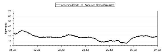
Figure 5-9 Measured vs. simulated flow for Anderson Grade, July 21-July 27, 2001
