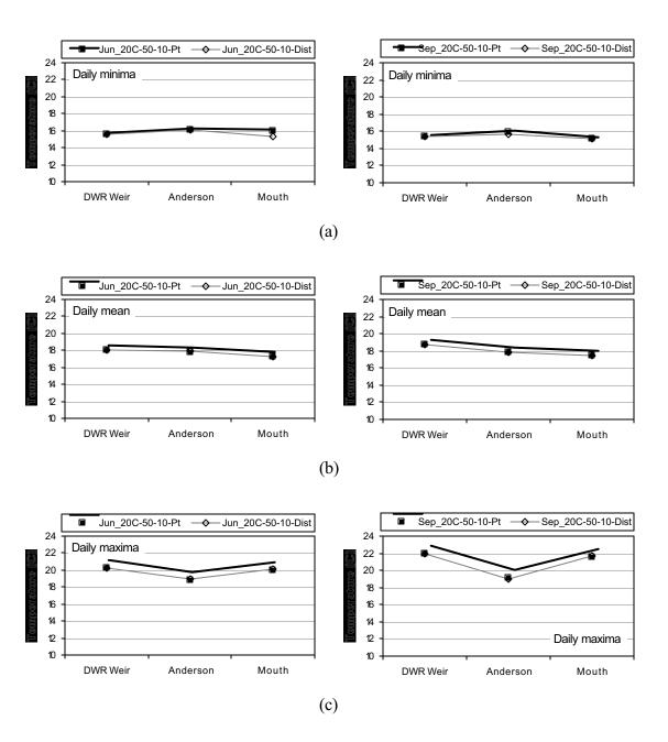
**Figure 5-38 Tailwater Return Study 20°C-50-10 results for June and September.** Upstream boundary condition of 20°C and 50 cfs at SRP, tailwater return flow of 5 cfs. Simulated (a) daily minimum, (b) daily average, and (c) daily maximum water temperature at DWR Weir, Anderson Grade Road, and the mouth of the Shasta River comparing point and distributed discharge of tailwater. Simulations designated by "month\_upstream water temperature-upstream inflow-tailwater flow" (e.g. Sep\_20C-50-10).
