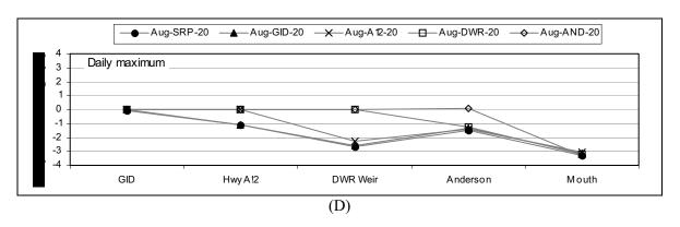
Figure 3.8: Flow regime results for 20 cfs inflows in August. Deviations from (A) August basecase condition in (B) daily minima, (C) daily average, and (D) daily maxima of simulated water temperature at GID, Hwy 12, DWR Weir, Anderson Grade Road, and the mouth of the Shasta River.
