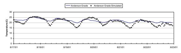
Figure 5-15 Measured vs. simulated temperature for Anderson Gr, Aug 17-23, 2001
