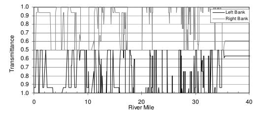
Figure 8. Longitudinal distribution of shade conditions on the Shasta River (tree height assumed 22 feet where present)
