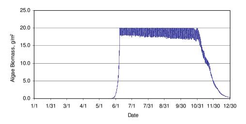
Figure 45. Algal biomass with global shade factor equal to 0.1
