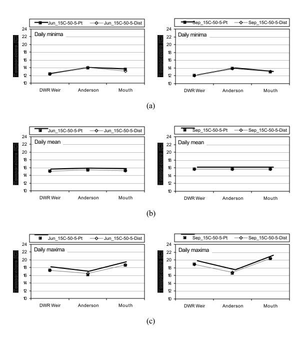
**Figure 5-33 Tailwater Return Study 15°C-50-5 results for June and September.** Upstream boundary condition of 15°C and 50 cfs at SRP, tailwater return flow of 5 cfs. Simulated (a) daily minimum, (b) daily average, and (c) daily maximum water temperature at DWR Weir, Anderson Grade Road, and the mouth of the Shasta River comparing point and distributed discharge of tailwater. Simulations designated by "month\_upstream water temperature-upstream inflow-tailwater flow" (e.g. Sep\_15C-50-5).
