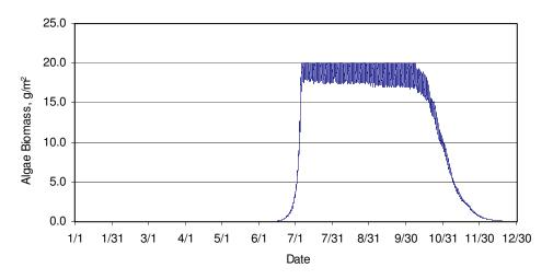
Figure 41. Algal biomass with maximum algal growth rate equal to 1.0 1/day
