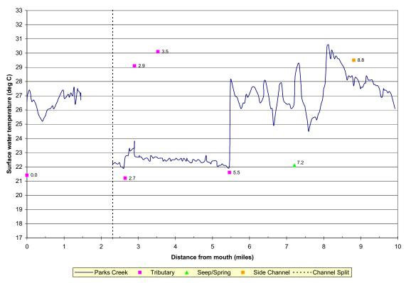
Figure 24 – Median channel temperatures versus river mile for Parks Creek.
