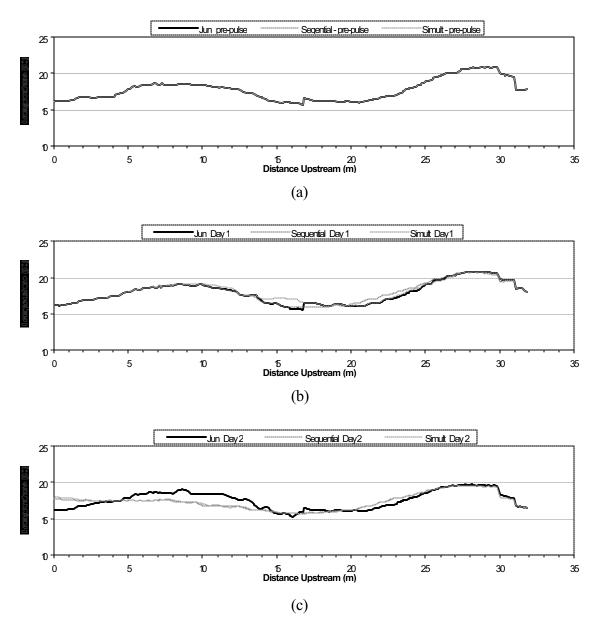
Figure 5-29 Longitudinal river temperature for June baseline, sequential, and simultaneous pulse flows: (a) pre-pulse, and representative (b) day 1 and (c) day 2 conditions.
