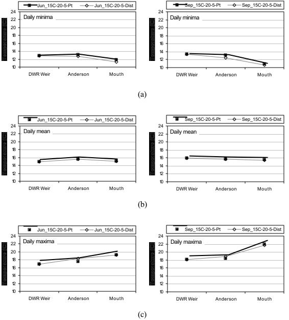
**Figure 5-31 Tailwater Return Study 15°C-20-5 results for June and September.** Upstream boundary condition of 15°C and 20 cfs at SRP, tailwater return flow of 5 cfs. Simulated (a) daily minimum, (b) daily average, and (c) daily maximum water temperature at DWR Weir, Anderson Grade Road, and the mouth of the Shasta River comparing point and distributed discharge of tailwater. Simulations designated by "month\_upstream water temperature-upstream inflow-tailwater flow" (e.g. Sep\_15C-20-5).
