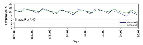
Figure 24. Temperature at Anderson Grade for 8/29/2002 – 9/04/2002
