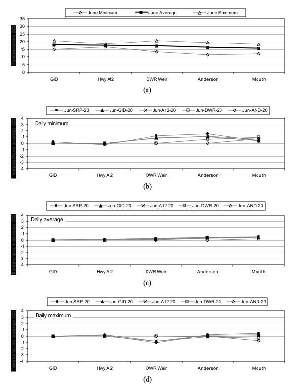
**Figure 5-24** Flow Regime Study results for 20 cfs inflows in June. Deviations from (a) June base-case condition in (b) daily minima, (c) daily average, and (d) daily maxima of simulated water temperature at GID, Hwy 12, DWR Weir, Anderson Grade Road, and the mouth of the Shasta River.
