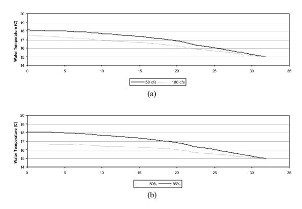
Figure 4-9 Longitudinal profile of average daily temperature for August 28, 2001 meteorological conditions flow vs. transmittance sensitivity (a) flow increased from 50cfs to 100cfs (b) transmittance decreased from 85% to 50%
