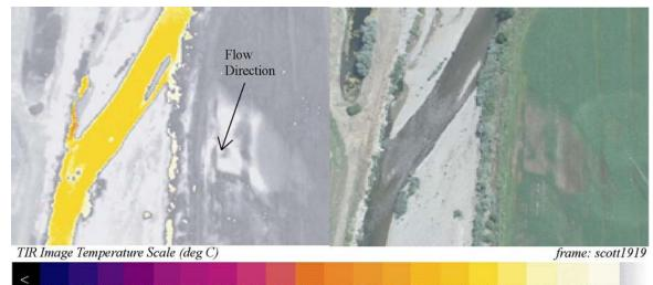
**17.0 17.5 18.0 18.5 19.0 19.5 20.0 20.5 21.0 21.5 22.0 22.5 23.0 23.5 24.0 24.5 25.0 25.5 26.0 26.5 27.0** Figure 8 – TIR/color image pair showing an example of a cool water seep detected at river mile 47.2 in the Scott River.
