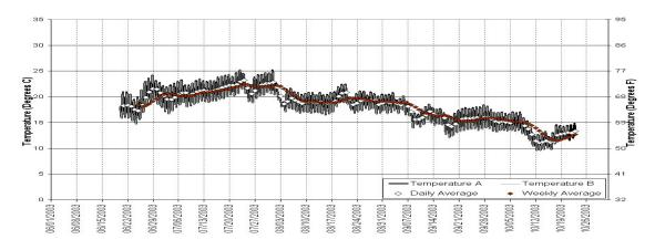
Figure 47. Continuous Temperature Data - Shasta River @ Freeman Road - Collected by NCRWQCB: 06/01/03 - 10/31/03. (For quality control purposes, two optic StowAway sensors ( A and B ) were deployed at this site).
