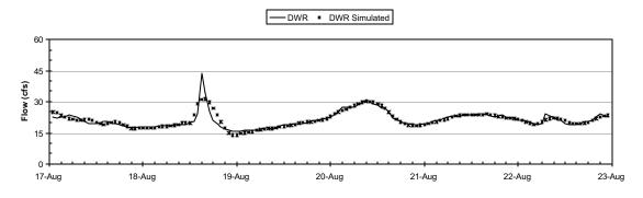
Figure 5-3 Measured vs. simulated flow for DWR Weir, Aug 17-Aug 23, 2001
