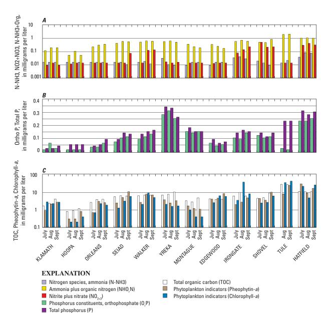
**Figure 10.** Monthly water-quality sampling data for July, August, and September 2002 for six sites on the Klamath River, one site on the Trinity River, three sites on the Shasta River, and two sites on the Lost River in the Lower Klamath River Basin, California. *A.* Nitrogen, *B.* Phosphorus constituents, and *C.* Total organic carbon (TOC), and phytoplankton indicators pheophytin-*a* and chlorophyll-*a*, calculated as concentrations.
