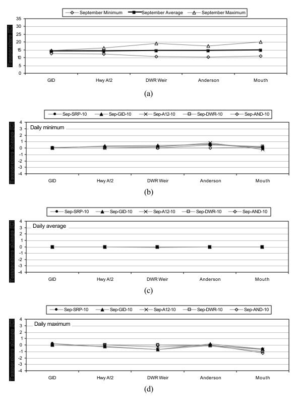
**Figure 5-27 Flow Regime Study results for 10 cfs inflows in September.** Deviations from (a) September base-case condition in (b) daily minima, (c) daily average, and (d) daily maxima of simulated water temperature at GID, Hwy 12, DW R Weir, Anderson Grade Road, and the mouth of the Shasta River.
