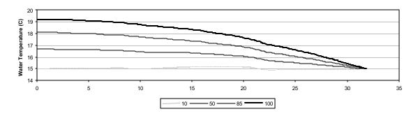
Figure 4-7 Longitudinal profile of average daily temperature for August 28, 2001 meteorological conditions for 50 cfs test case with varying transmittance (10%, 50%, 85%, 100%)
