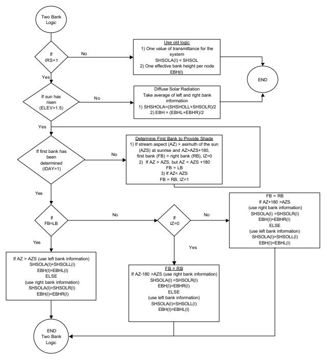
Figure 2-6 Flowchart of two-bank shading logic
