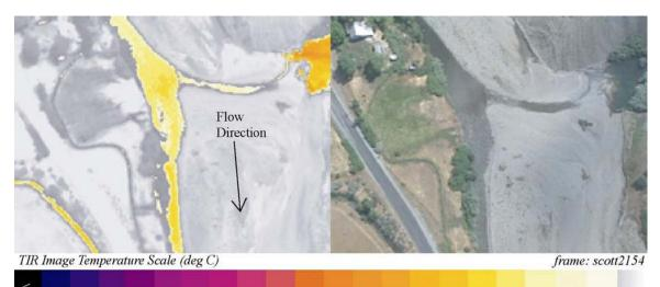
**17.0 17.5 18.0 18.5 19.0 19.5 20.0 20.5 21.0 21.5 22.0 22.5 23.0 23.5 24.0 24.5 25.0 25.5 26.0 26.5 27.0** TIR/color video image pair showing cool surface water in the mine tailings near the Scott River (25.3 °C) at river mile 53.1.
