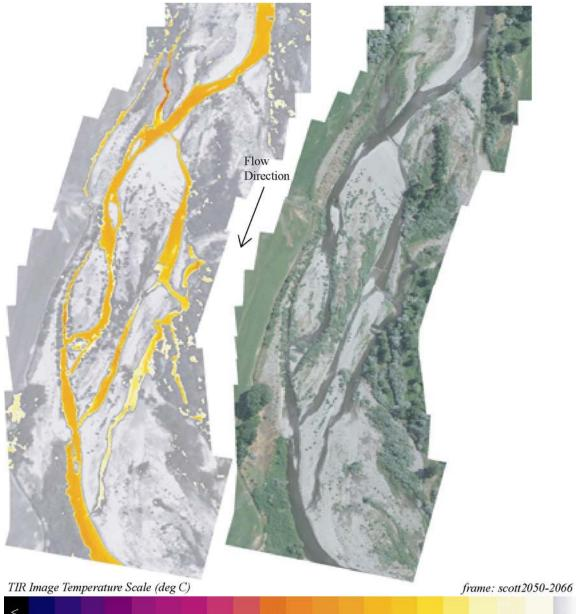
**17.0 17.518.0 18.5 19.0 19.5 20.0 20.5 21.0 21.5 22.0 22.5 23.0 23.5 24.0 24.5 25.0 25.5 26.0 26.5 27.0** TIR/color video image pair showing a warm side channel on the left bank (bottom portion) and a spring/seep  $(21.4 \,^{\circ}\text{C})$  on the right bank (top portion) of the Scott River  $(23.4 \,^{\circ}\text{C})$  at river mile 51.0.
