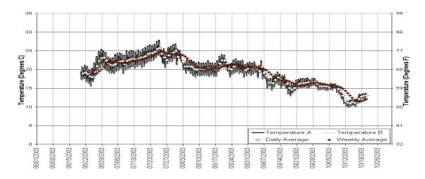
Figure 48. Continuous Temperature Data - Shasta River @ Yreka-Ager Road - Collected by NCRWQCB: 06/01/03 - 10/31/03. (For quality control purposes, two optic StowAway sensors ( A and B ) were deployed at this site).
