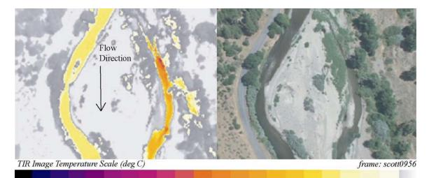
**17.0 17.5 18.0 18.5 19.0 19.5 20.0 20.5 21.0 21.5 22.0 22.5 23.0 23.5 24.0 24.5 25.0 25.5 26.0 26.5 27.0** TIR/color video image pair showing a spring/seep emerging from within the left bank channel of the Scott River (25.3 °C) at river mile 24.5.
