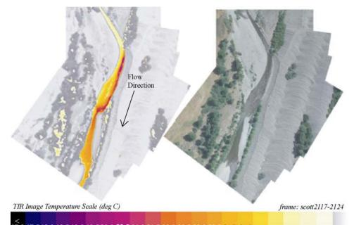
**17.0 17.5 18.0 18.5 19.0 19.5 20.0 20.5 21.0 21.5 22.0 22.5 23.0 23.5 24.0 24.5 25.0 26.5 27.0** Figure 7 – TIR/color image mosaic showing a sub-surface discharge which appears to emerge from mine tailing along the left bank and decreases water temperatures in the Scott River by  $\approx 3.0^{\circ}$ C at river mile 52.3.
