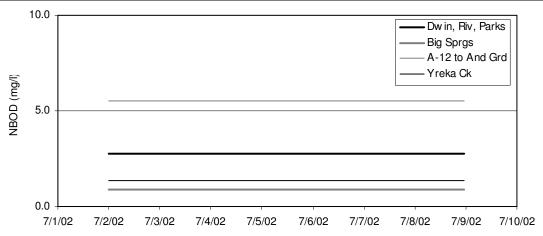
Figure 12. NBOD boundary conditions for the July, August-September, and September calibration periods (same for all periods, only July presented)
