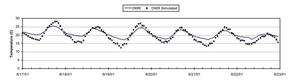
Figure 5-14 Measured vs. simulated temperature for DWR Weir, Aug 17-23, 2001
